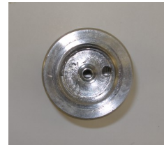
Figure 3: Valve body. Debris around the center hole may lead to valve malfunction.
