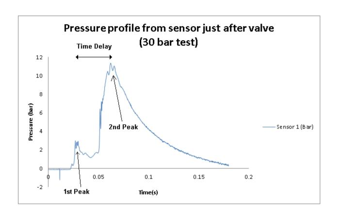
Conditions: High pressure air on one side (upto 30 bar) and water on other side (at 1 bar).
